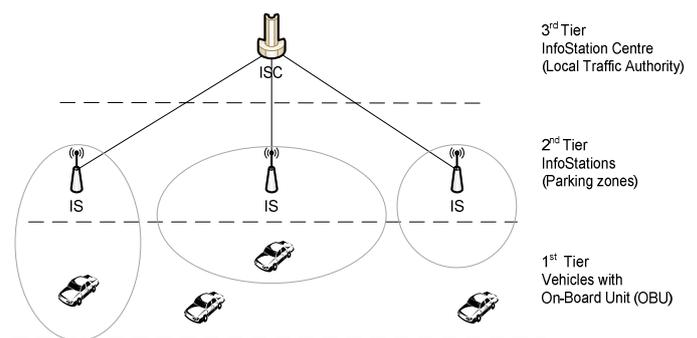
Figure 2. Three-Tier System Network Deployment
