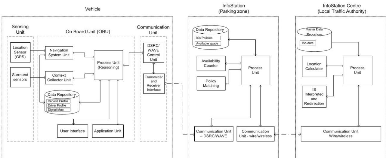
Figure 3. On-street Parking System Architecture
