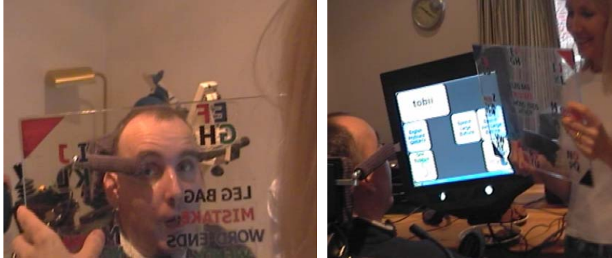
Figure 7. Michael using his E-tran frame, and using eye gaze, on-screen keys and the E-tran together to communicate
