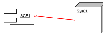
Deployment Diagram Showing the Interface relationship between source code file, SCF1, and file device, Sys01
